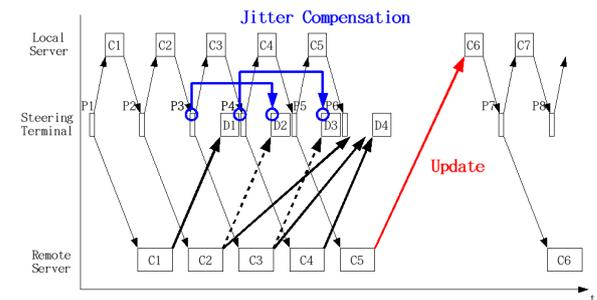
Figure 2: Cooperation of the Local and Remote Servers in Simulation Caching.
